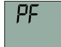
Battery total empty
